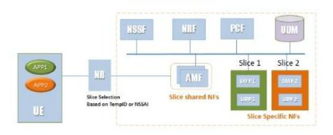
Through PCF, 5GC can customize NSSP (Network Slice Selection Policy) for different APPs of the UE, and deliver it to the UE, such as WeChat -> eMBB, meter reading application -> mMTC, and V2X application -> URLLC.
