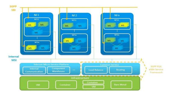
cloud native technology/. It decouples an NE into a group of independent NFs, and each NF is decoupled into multiple NF Services. In addition, in the eSBA stage of 3GPP R16, NFs will decouple into more and smaller NF Services. Therefore, to better adapt to different service scenarios and vertical industries, it is the best choice to construct SBA+ 5GC with Cloud Native technology such as micro-service NF.
