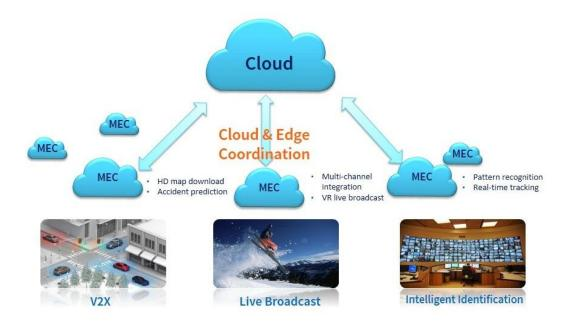
Therefore, it is necessary to set up a local distributed network at the end that is close to data to provide computing and storage capabilities, improve the performance and reliability of applications, reduce the load of the core network, and focus on edge computing. Operators can use edge computing to significantly improve user experience, reduce network transmission load, reduce response delay of devices and systems, and improve control accuracy.
