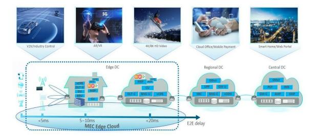
5GC has a natural attribute of CUPS, driving the cloud network evolving to the distributed cloud architecture. By building a 5G-oriented distributed cloud architecture, the user plane is moved to edge nodes and is deployed in combination with the MEC platform, effectively extending cloud computing power from the center to the edge to implement fast service processing and proximity-based forwarding, so as to meet diversified application scenarios of 5G.
