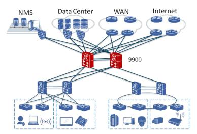
The ZXR10 9900/9900-S Series switch works as high density 10GE/40GE aggregation switch which provide 40GE/100GE as uplink in carrier network. Through L2/L3 features and carrier-class reliability, the ZXR10 9900/9900-S Series switch transmits the traffic from the aggregations and forward it to the routers. VSC2.0 technology can realize fast switchover when failure happens.
