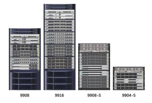
Coupled with distributed ROSng Software Platform, the ZXR10 9900/9900-S Series switch has models as 9908, 9916 (8 Switch Fabric Unit Slots) and 9904-S, 9908-S (4 Switch Fabric Unit Slots). The ZXR10 9900 Series switch delivers comprehensive products:
