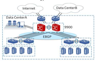
The ZXR10 9900/9900-S Series switch works as Core switch on a typical data center network. The ZXR10 9900/9900-S Series switch has high-density 40GE/100GE interfaces to aggregate the TOR switches and interconnects to the backup data center core switches or the routers through 100GE interfaces. Deploy EBGP and VSC2.0 technology to build a non-blocking Layer 3 network, which allows large-scale VM migrations and flexible service deployments.
